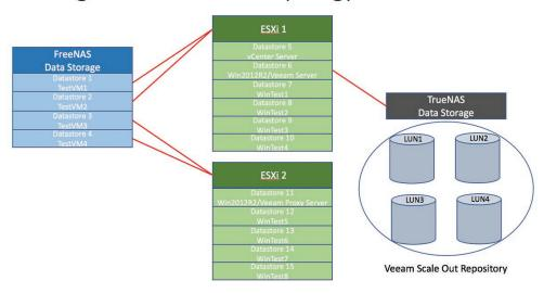
The FreeNAS All-Flash Array has four LUNs, each LUN presented to an ESXi server as an iSCSI datastore and dedicated to one each of the four 100 GB test VMs. Two of the test VMs are running on ESXi Server 1, and the other two test VMs are running on ESXi Server 2.
